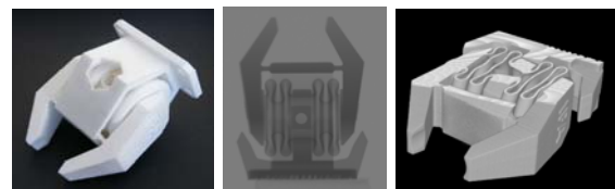
Figure 2: Photo of gripper (left), 2D-X-ray image (middle), cutted voxel model (right)
