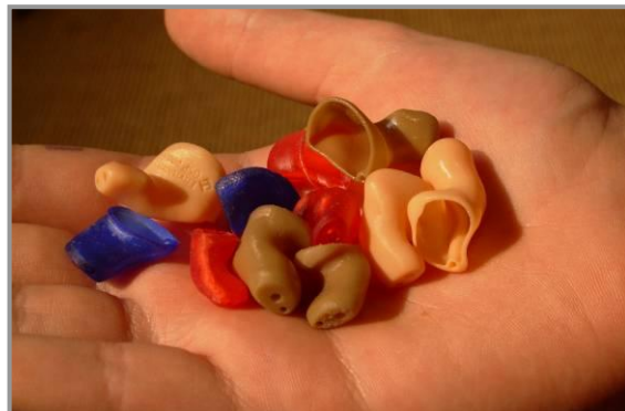
Figure 1 - Personalised RM hearing-aid shells produced using Envisiontec Perfactory
