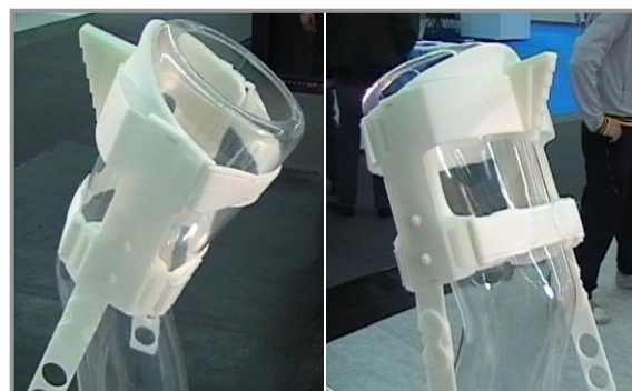
Figure 4 – personalised 'knee-brace' manufactured using Selective Laser Sintering
