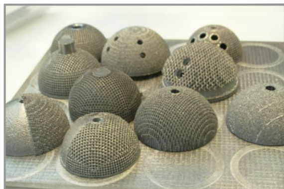
Figure 3 – Accetabular cups manufactured using ARCAM Electron Beam Melting
