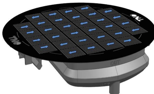
Fig. 18 Thermal stabilised table by means of free form cooling structure (source TNO)
